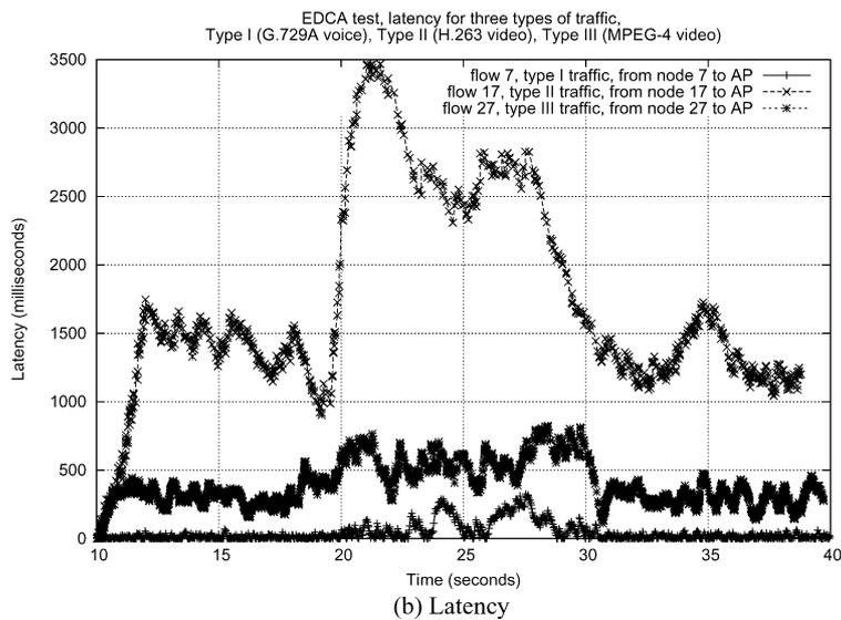
Figure 8. Throughput and latency for EDCA tests.
