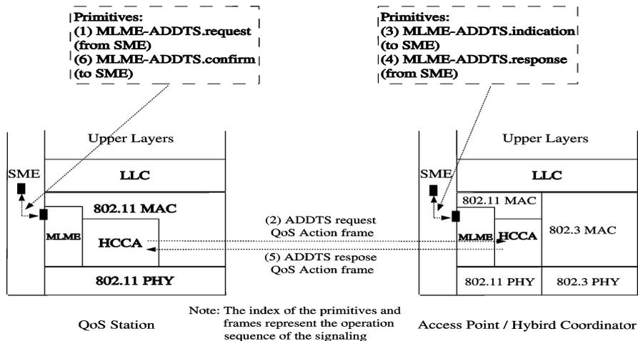
Figure 5. Signaling for adding a TS in 802.11e HCCA mode.
