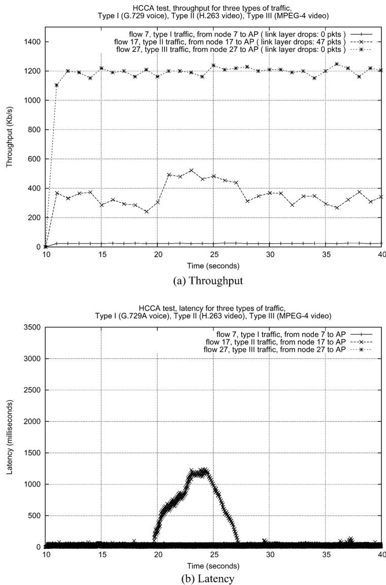
Figure 9. Throughput and latency for HCCA tests.
