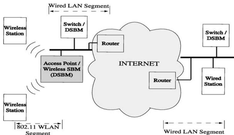
Figure 4. An end-to-end QoS architecture with wireless SBM.
