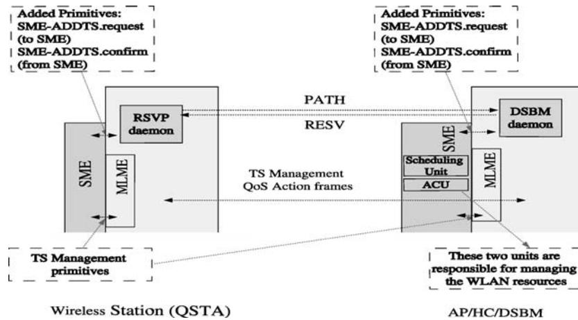
Figure 7. Synchronization of 802.11e signaling with RSVP/SBM for case 1.
