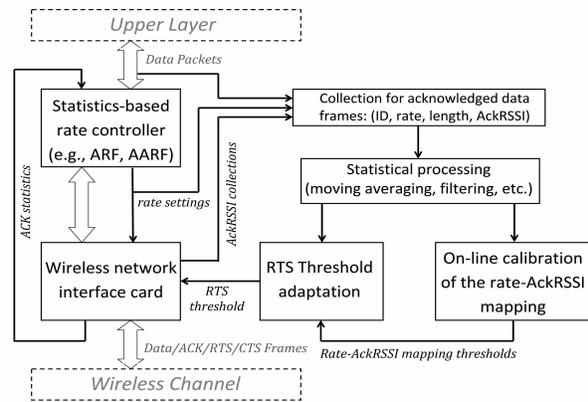
**Figure 2. The RADAR rate adaptation system**
