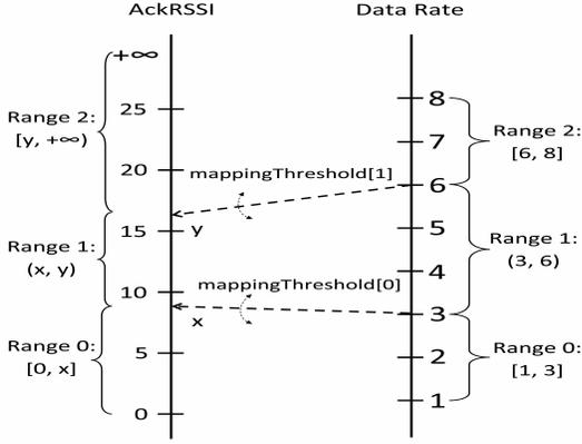
**Figure 3. The dynamic mapping between rate and AckRSSI ranges**
