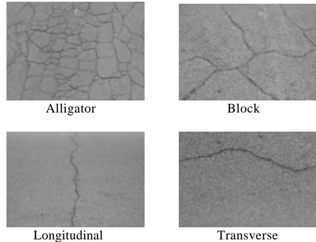
Figure 1.1 Types of pavement cracks
