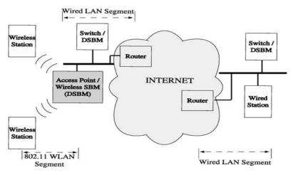
Figure 4. An end-to-end QoS architecture with wireless SBM.
