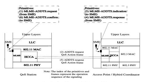
Figure 5. Signaling for adding a TS in 802.11e HCCA mode.
