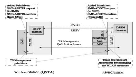
Figure 7. Synchronization of 802.11e signaling with RSVP/SBM for case 1.
